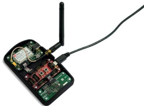
Mobile Bluetooth Low Energy gateway prototype developed by Oberon microsystems
