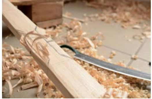
The drawknife ( Ziehmesser ), partly visible in the background, is a typical bowyer's tool. It is often the first tool used to give a plain stave the first look of a bow.
